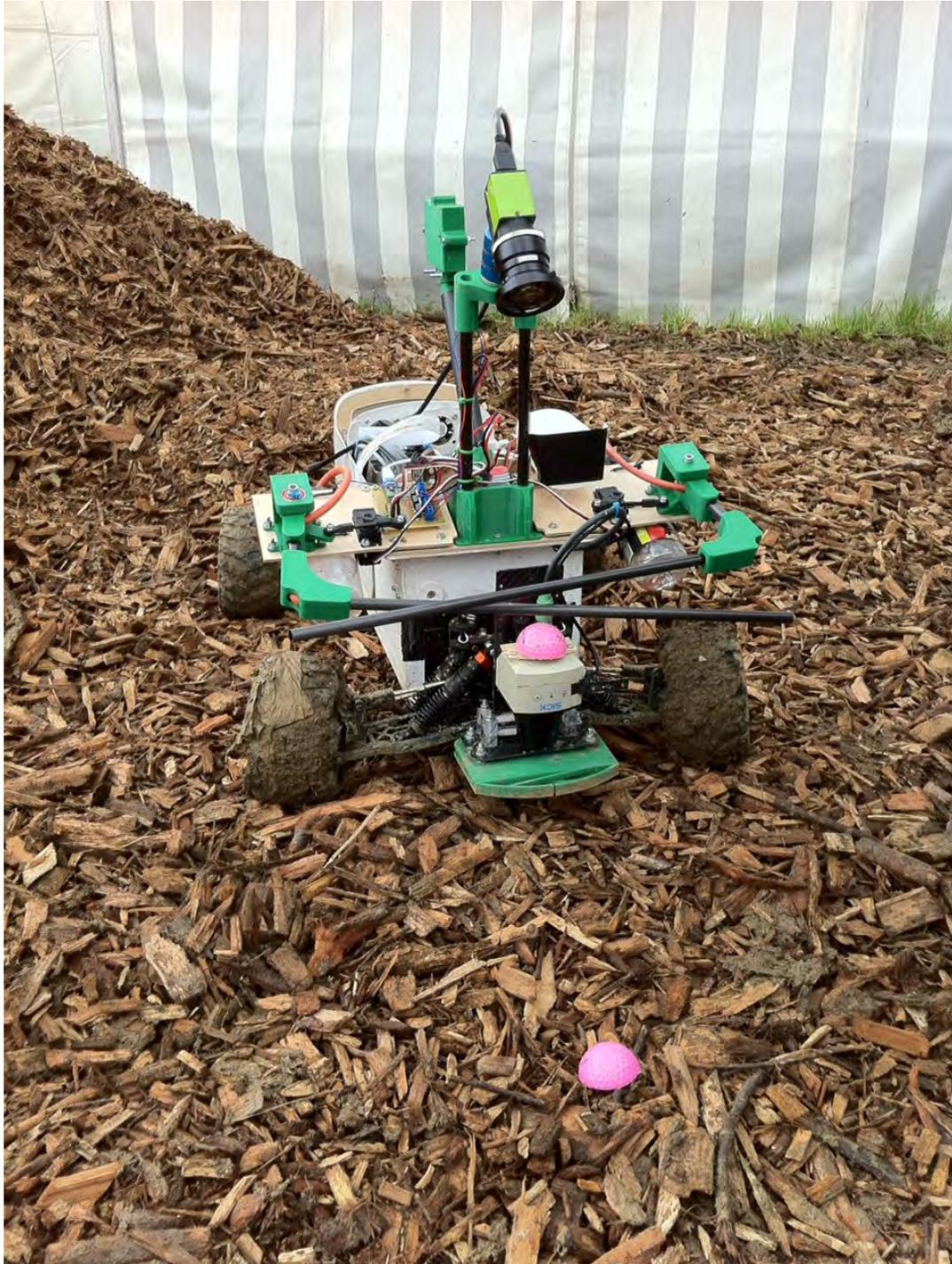
Another feature of our construction are various 3D printed parts which were used for different tasks like the affixing of sensors etc. (all green parts in the picture, except the
