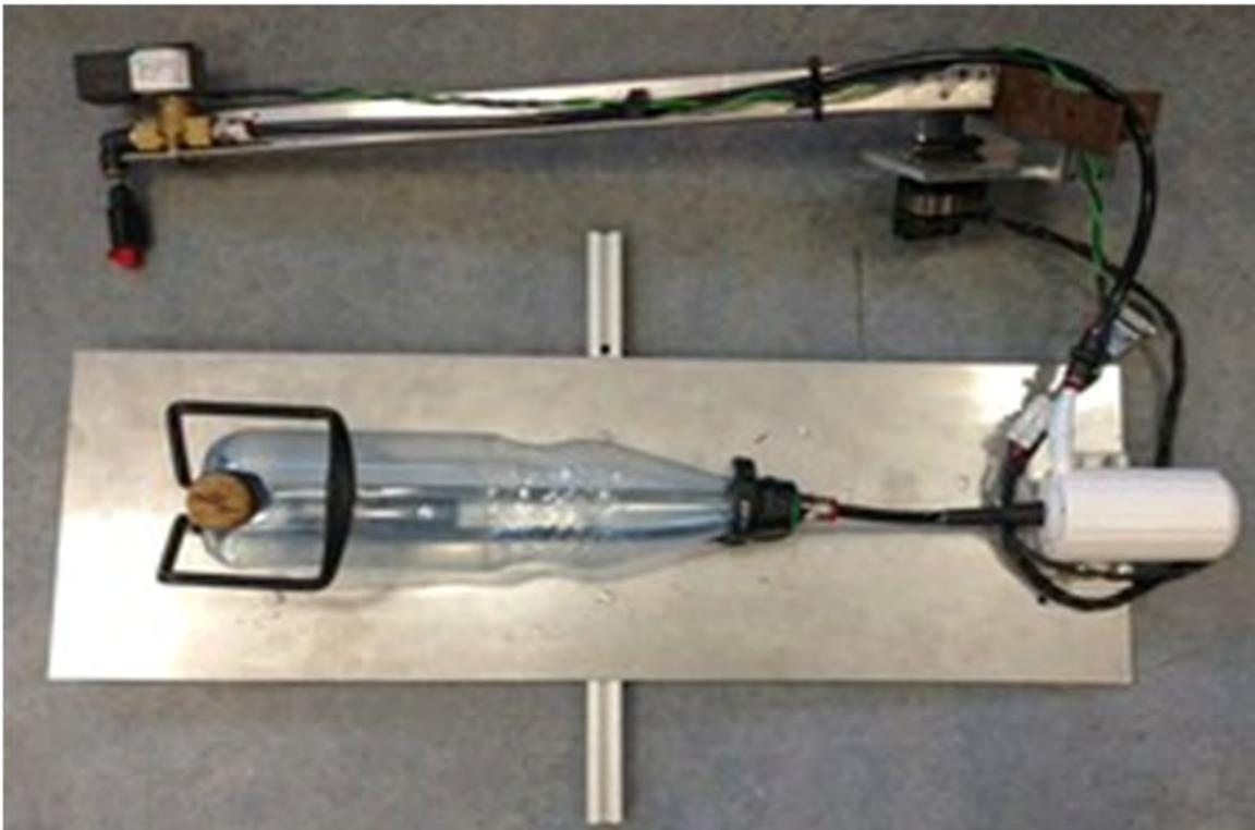
Fig. 6: Sprayarm and water pump with container
