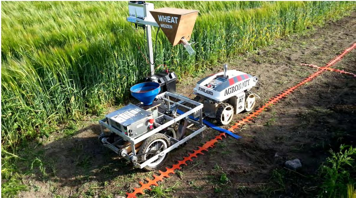
Figure 28. The robot performing the seeding task in Finland in June after the Field Robot Event. The robot is driving to the filling station. Here, the orange tape is used instead of the red used in the competitions.
