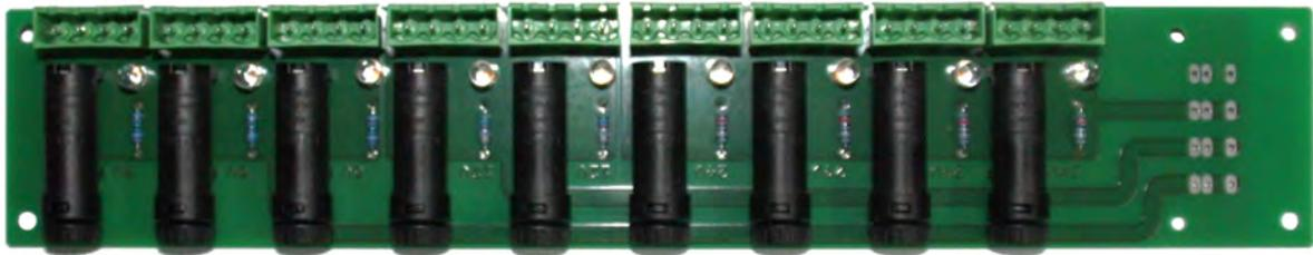
Figure 5: Fuse board
