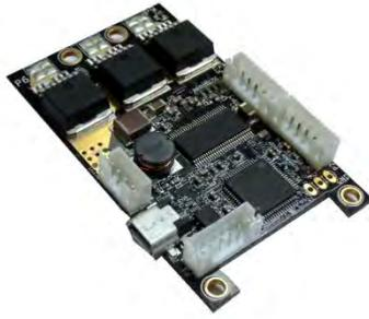
Figure 9. VESC, the motor controller used in the axle modules.
