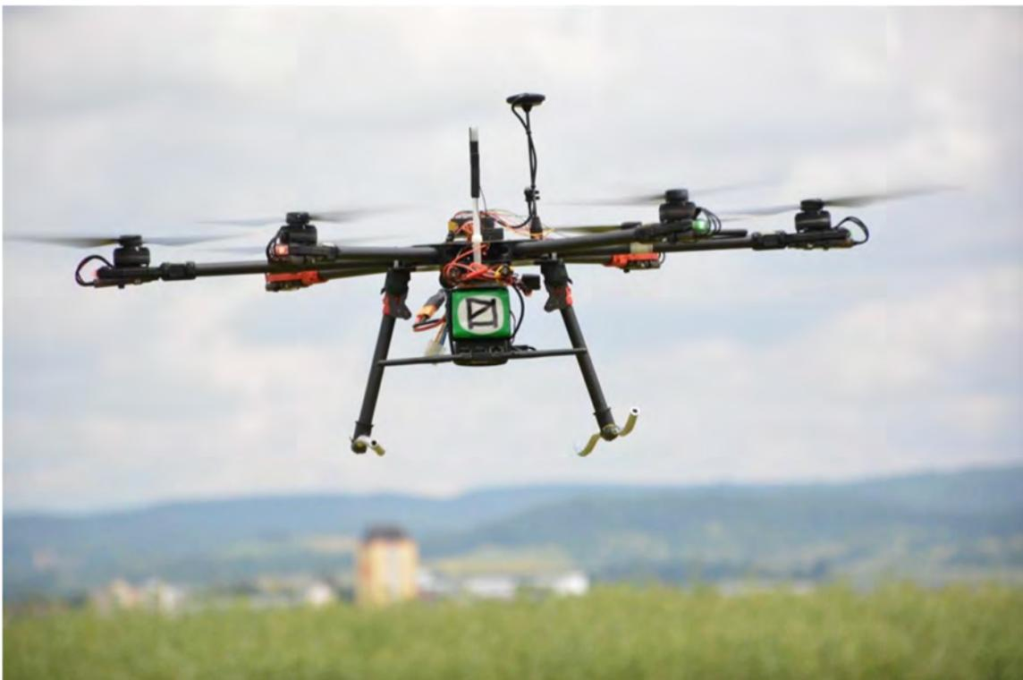
The drone consists of three phase motors, ESCs (electronic speed controllers), propellers, flight controller, receiver and a battery of 10 Ah (6s).
