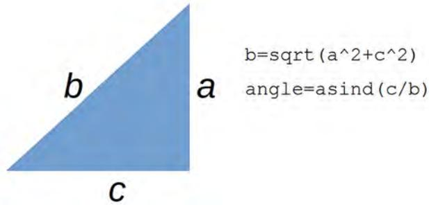
Where  $c$  is the ball location relative to the robots y-axis and  $a$  is the servo height. The angle between  $a$  and  $b$  is the servo angle needed to aim the spray towards the detected ball.
