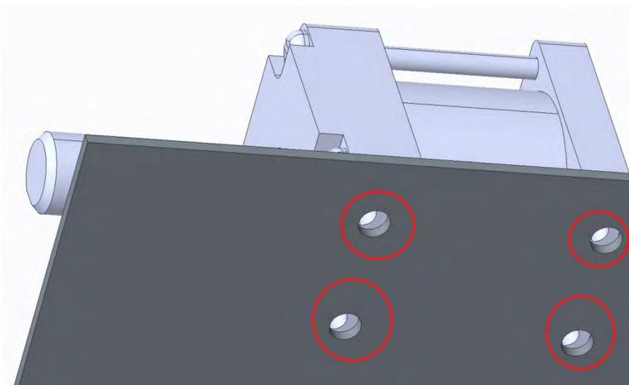
Figure 3. Banebots gearbox and axle module wall. Red circles indicate the misalignment of the holes on wall and gearbox
