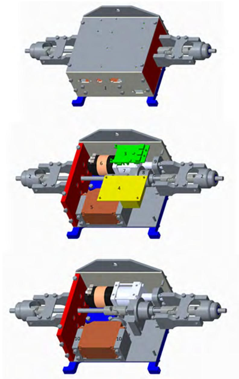
Figure 1: Breakdown of an axle module with its main components numbered.
