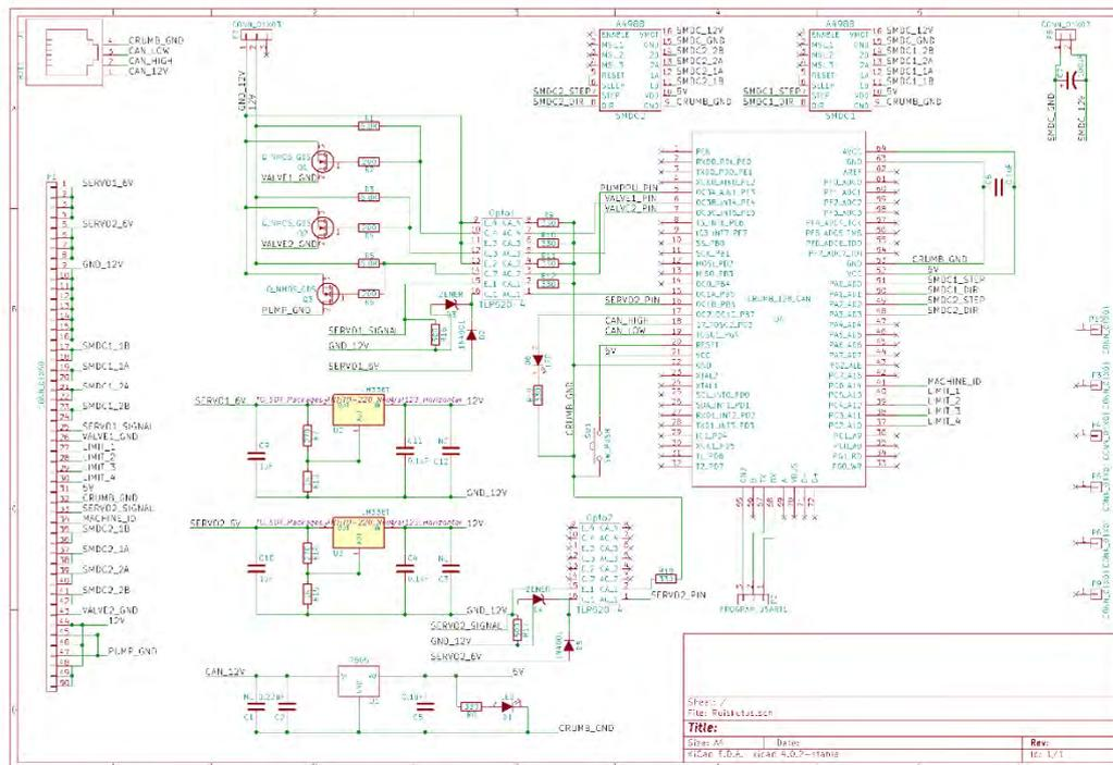
Figure 20. Schematic of the main printed circuit board for the egg collector and weeding device.
