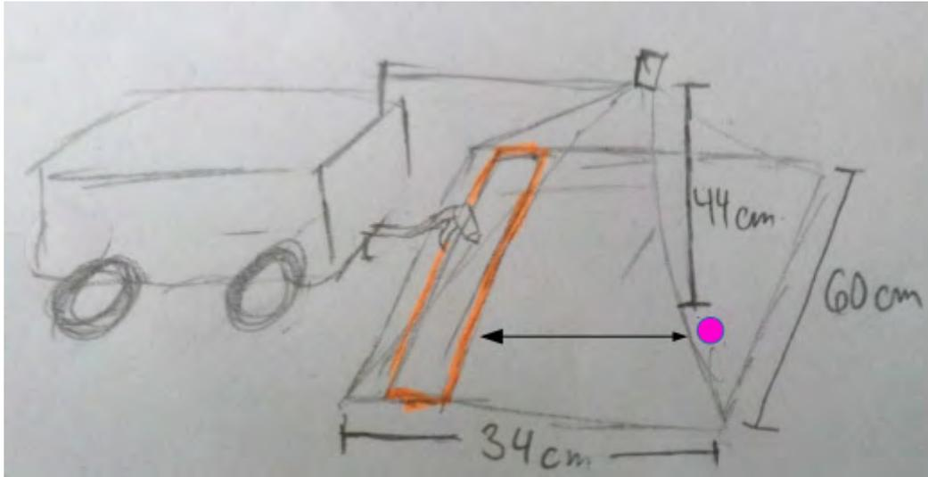
Figure 1 shows a sketch of the robot's spraying setup without the sirene. The orange area is the spray range. The robot has to approach the ball until the ball is within this area in order to successfully spray.
