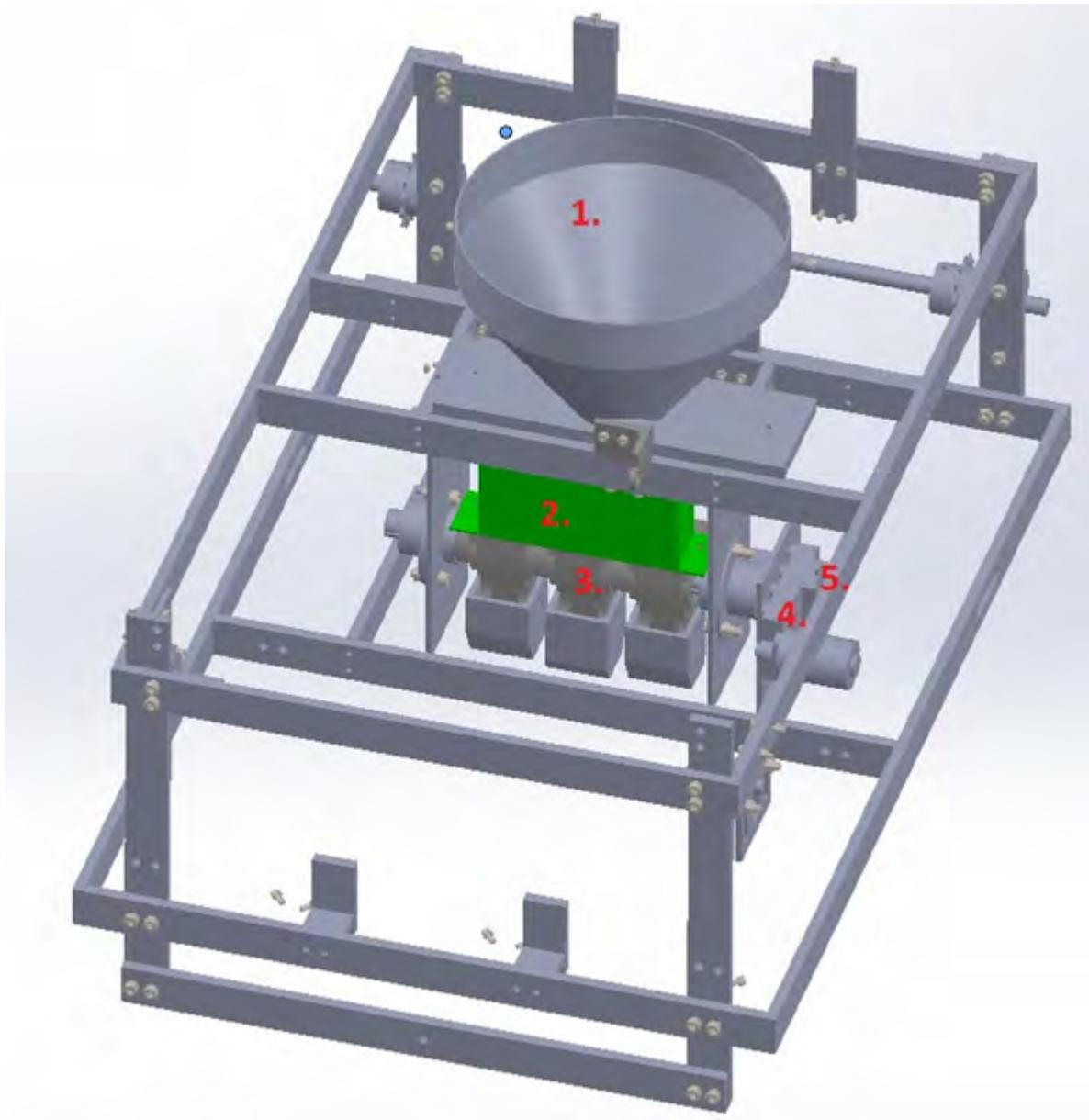
Figure 24. 3D model for seeding system in trailers body. (Seeding pipes not shown in figure) parts: part 1: funnel, part 2: Seed separator, part 3: Seeding units, part 4: 12 V dc motor, part 5: Encoder.
