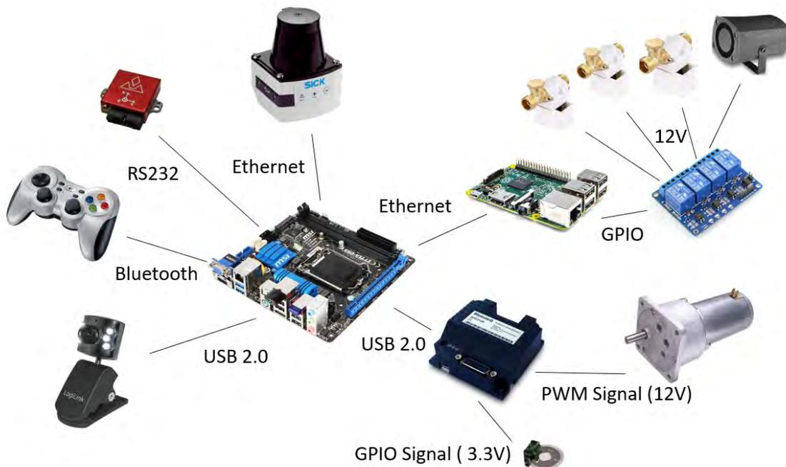
Figure 3: Signal flow diagram showing the general setup of the used robot components
