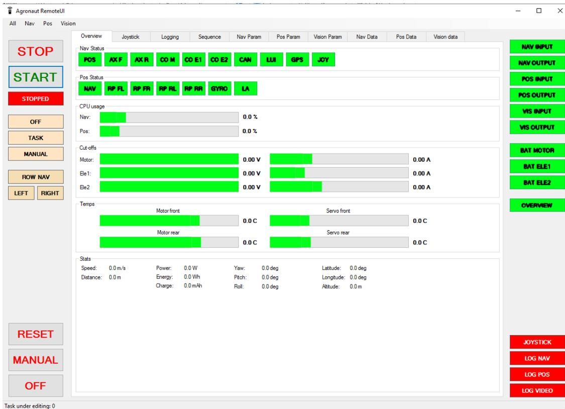
Figure 10. The main view of the RemoteUI window. This view represents the most significant information of the state of the robot.
