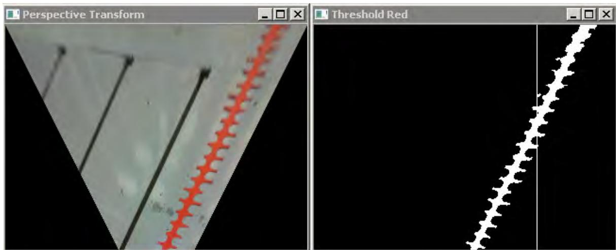
Figure 31. This figure represents the detection of the longitudinal red line. The line is skewed but the algorithm finds the mass centrum which is represented by the thin white line.
