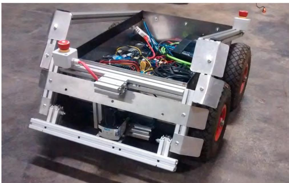
Figure 1: Robot Talos in the raw setup with open lid and Sick laser scanner attached
