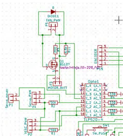
Figure 4: Optocoupler annotated Opto1, power and actuator connectors
