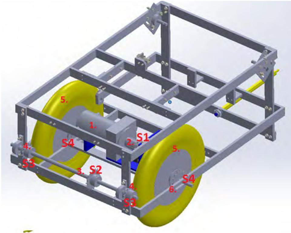
Figure 23. 3D model from Transmission in trailer (chains not in picture) parts: part 1: motor (ATV 900), part 2: Bike's rear hub, part 3: Countershaft, part 4: Sprocket wheel, part 5: tyre, part 6: bit for straining chains, S1-S4 Sprocket wheels.
