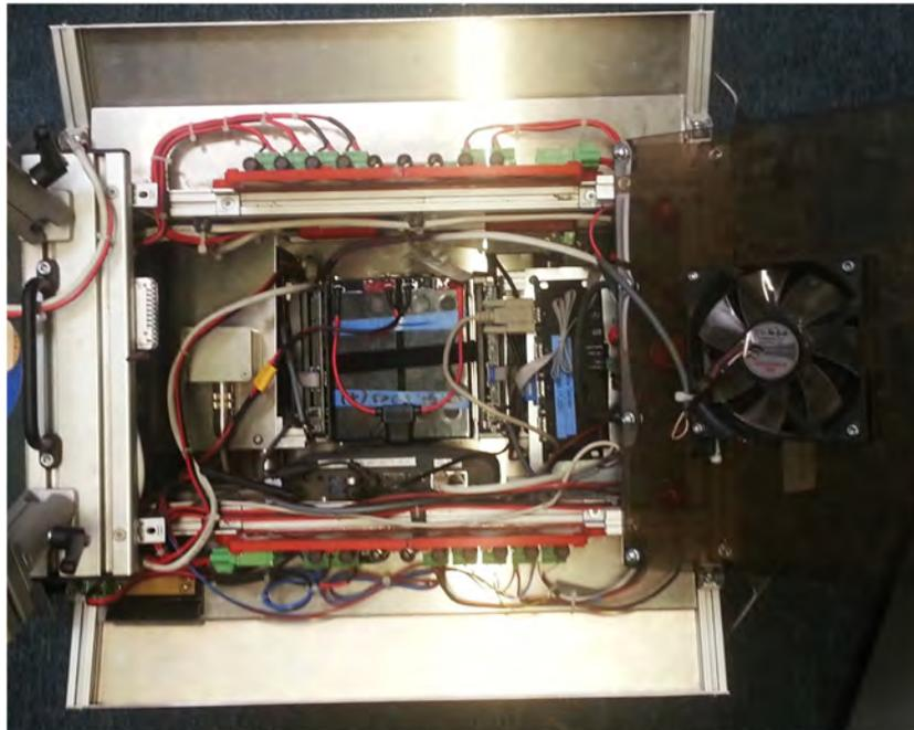
Figure 3: Inner assembly of the robot
