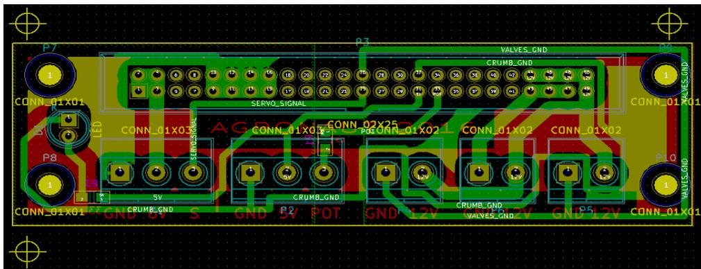
Figure 21. Printed circuit board design of the sprayer devices dedicated board.
