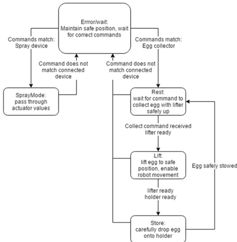
Figure 22. The state machine of the egg collector and weed spraying microcontroller
