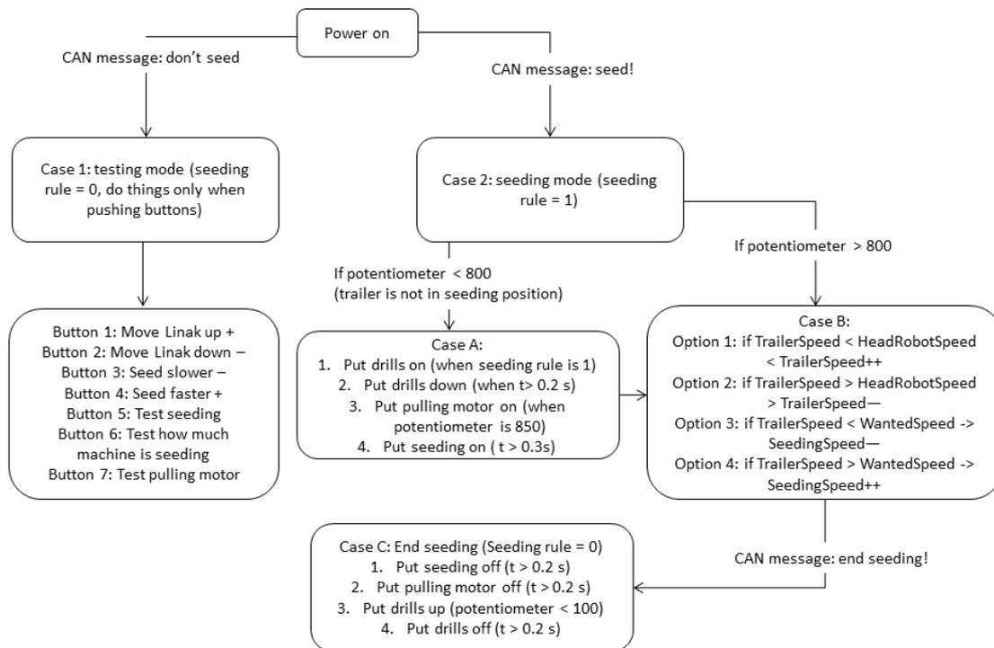
Figure 27. One of the optional state machines of the trailer software.
