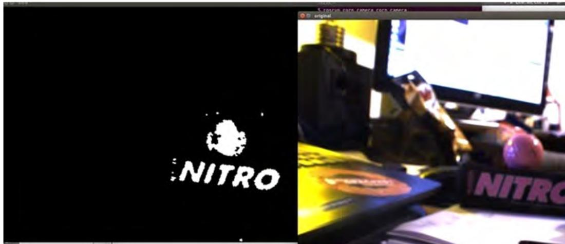
**Fig. 4.** An example of colour segmentation; original image on the right and its binary representation on the left.
