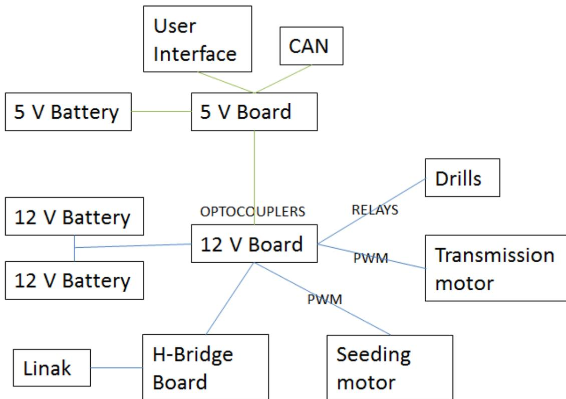
Figure 26. The general schema of the electrics of the trailer
