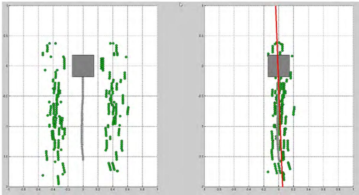
Figure 13. On the left, the gray box represents the robot and the gray dots the path of the robots. RangePack measurements as aside of the robot and represented by the green dots. On the right, the measurements are moved towards the center. The red line represents the estimated center line between the rows.
