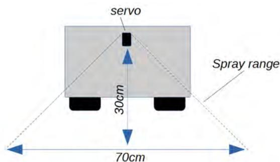
Having the ball’s location on the 70 cm stripe and the height of the servo, an angle for the servo can be calculated using:
