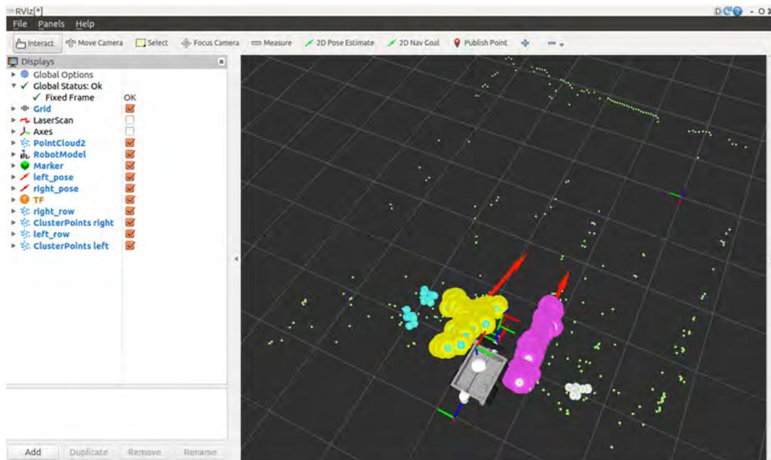
Figure 6: robot model, Point clouds and resulting line directions
