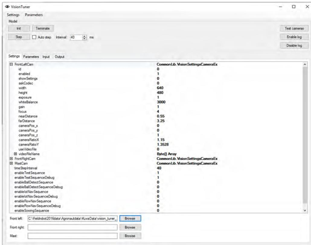
Figure 11. The VisionTuner software window. The VisionTuner contains all the parameters and setting for tuning the machine vision.
