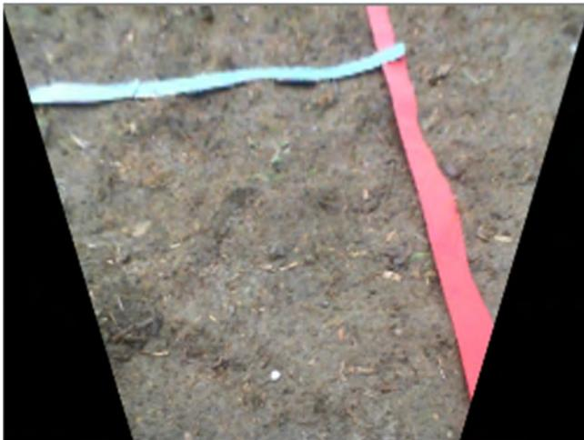
Figure 16. Camera view after inverse perspective mapping.
