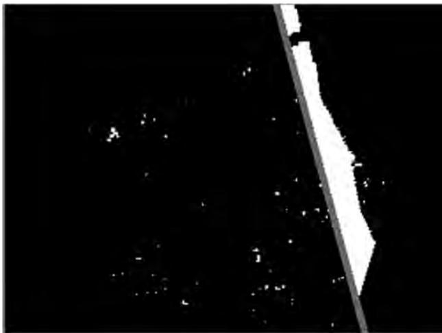
Figure 17. Image without filters (but with one Hough line showing) after red ECCRI color transform and thresholding
