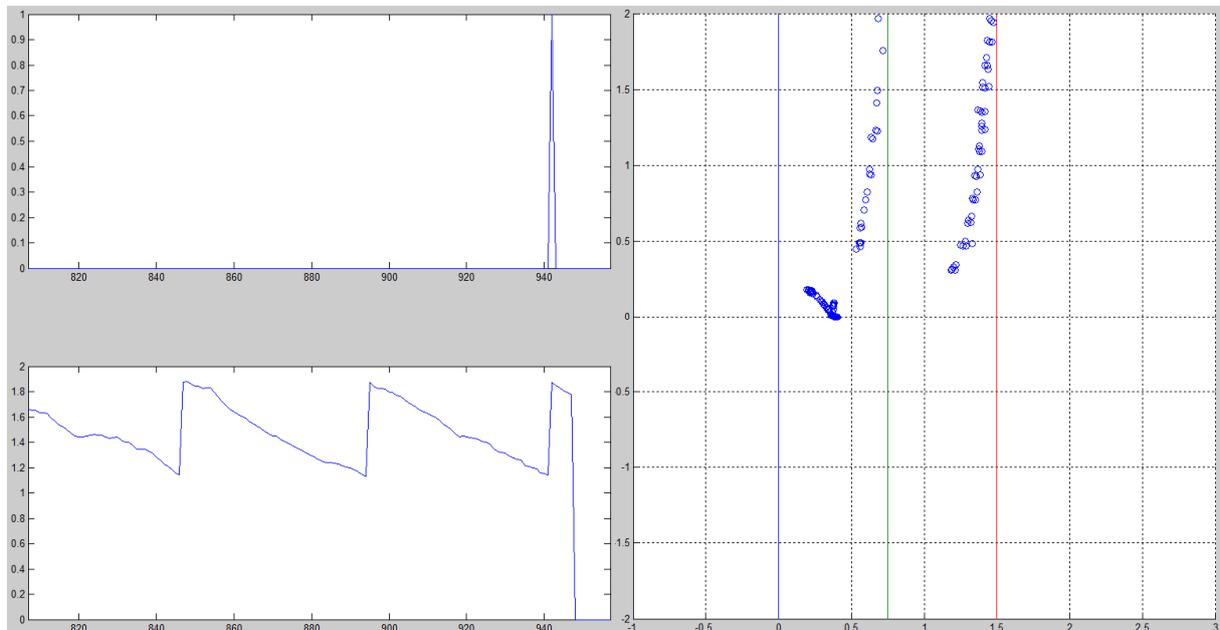
Figure 15. The blue circles represents the measurements from the laser scanner. The blue vertical line represents the level of the center of the robot. The algorithm keeps tracking the free space between the maize rows. When a row passes the level of the robot, a row is considered being passed. The algorithm begins to track the next free space. In this example the robot attempts to turn to the fourth row spacing. The impulse-triggering robot to turn back to row is seen in the up-left plot.
