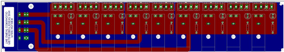
Figure 4: PCB-design of the fuse boards
