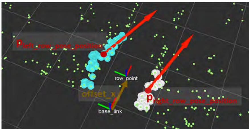
Figure 5: description of the rows and the resulting row point. The base\_link coordinate system corresponds to the robot center.
