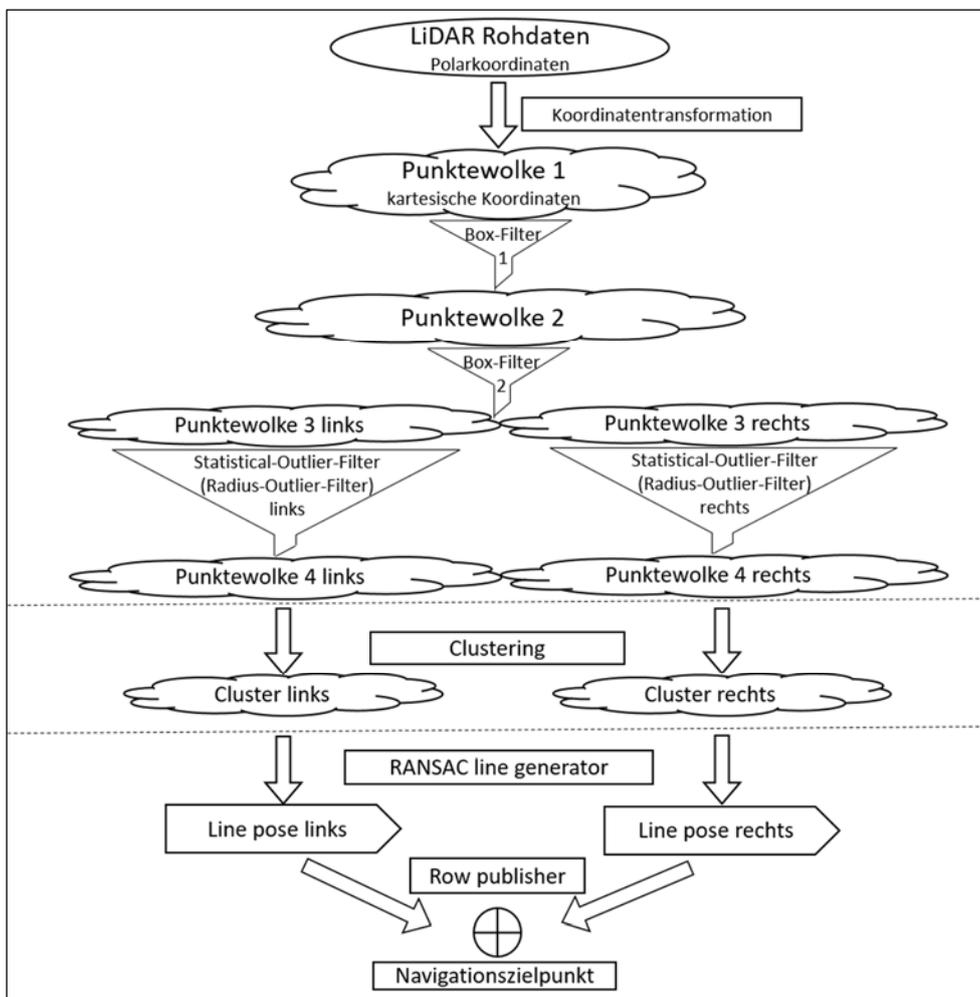
Figure 4: Description of the filtering algorithm used for the Field Robot Event
