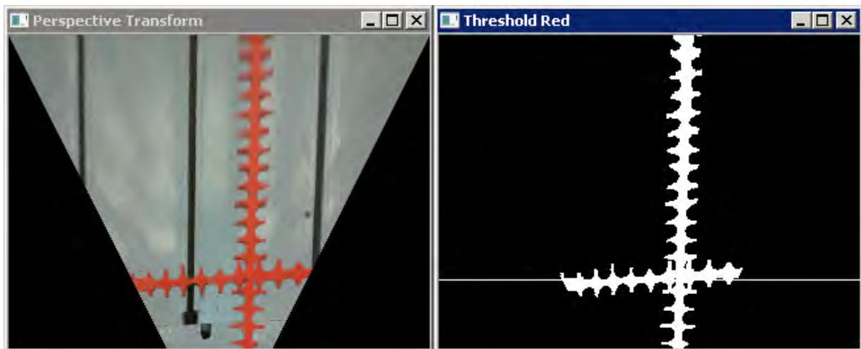
Figure 30. The machine vision detects the transverse red line and the estimated result is represented as the thin white line.
