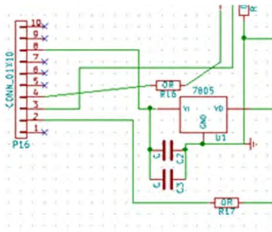
Figure 5: 10 pin header and voltage regulator
