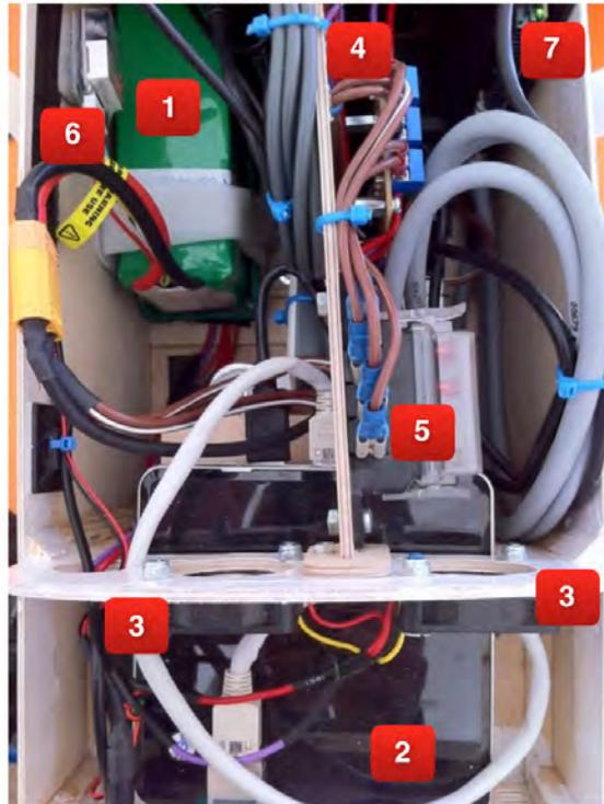
(1): 16 Ah LiPo Accumulator, (2): Intel NUC-Computer with Ubuntu-Linux, (3): small fans, (4): power distributor, (5): circuit board with several fuses, (6): LiPo safer, (7): Epos-Motorcontroller
