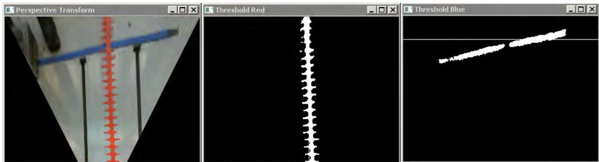
Figure 29. The machine vision algorithm for the seeding task. The first image is being perspective transformed. In the center the red color is thresholded as well as the blue color in the right image. In the right, the thin white line presents the measurement result.
