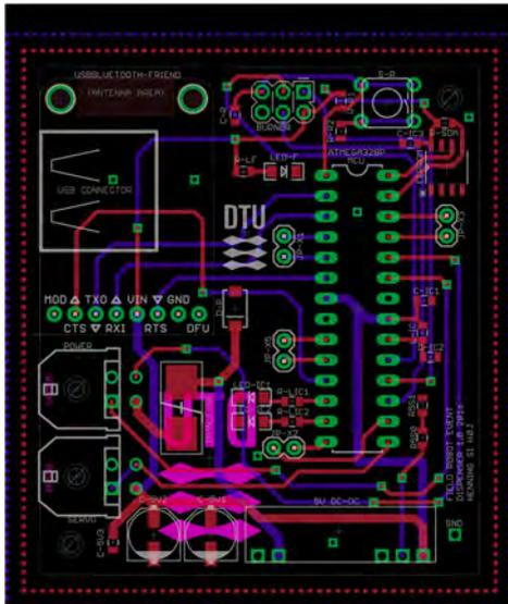
This board allows a smartphone to control the servo motor through a USB or bluetooth connection. The smartphone can then connect to the internet, and check for dispense-request on a server.
