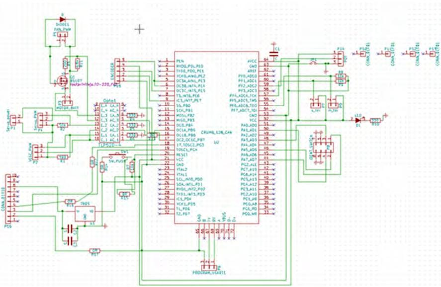
Figure 6. Schematic of the printed circuit board for the axle modules
