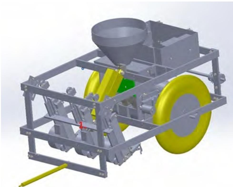
Figure 25. 3D model showing the drill rig halfway between working and transportation stance. Parts: Part 1 Drill holder.
