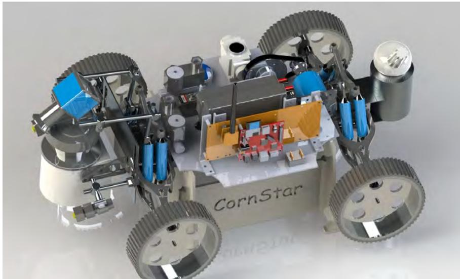
**Fig. 1.** Render of the Constar robot.
