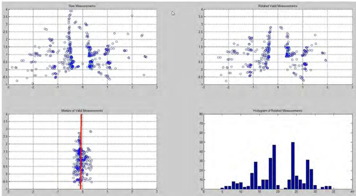
Figure 14. The raw laser data represented in up left is being rotated (up right) and the histogram of the rotated data is seen in down right. Once the optimal rotation is being found, a modulo is taken (bottom left). The remaining data is being used to find the final estimate for the center line between the rows (the red line).
