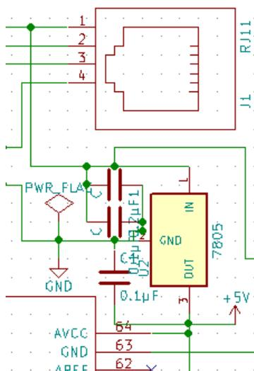
Figure 7. Schematic of the design of decreasing voltage from 12 V to 5 V.
