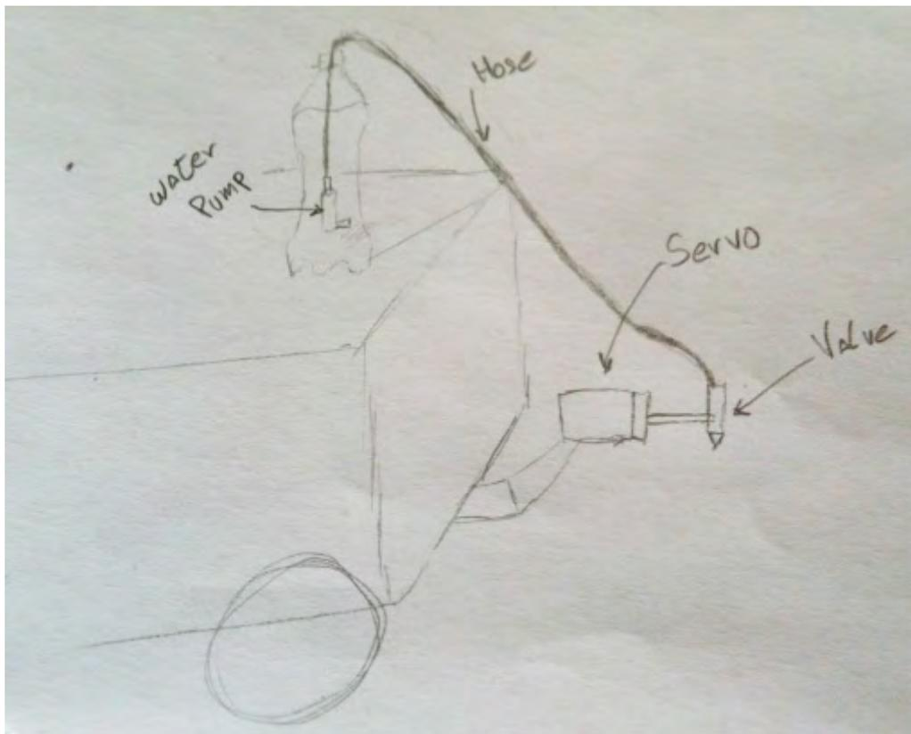
Figure 2 shows in detail the connection of the water to the nozzle (valve)
