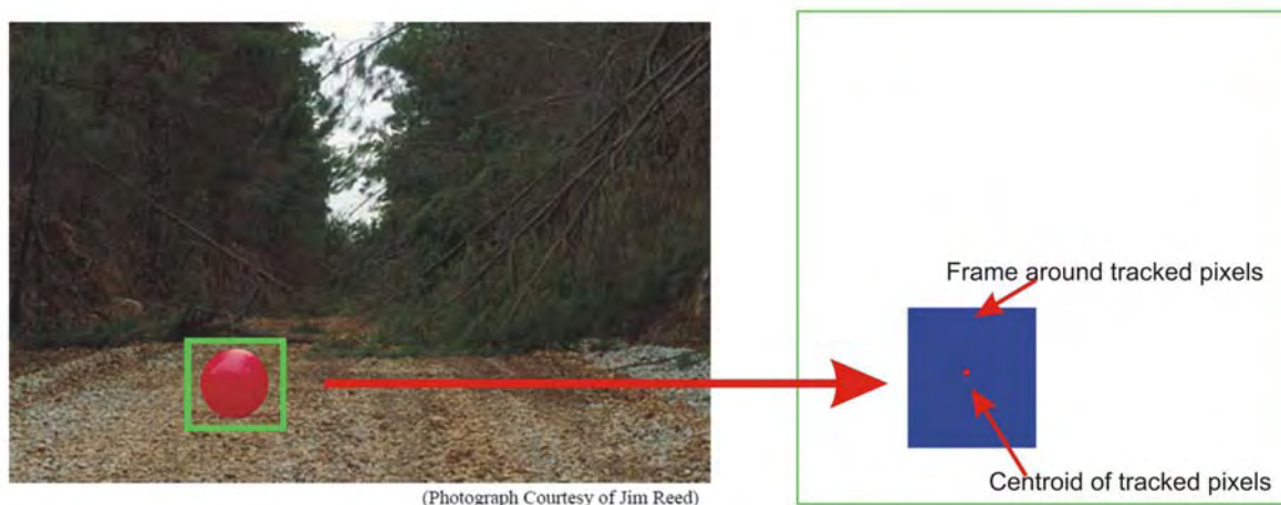
Fig. 7: Colour-tracking of the CMUcam2
