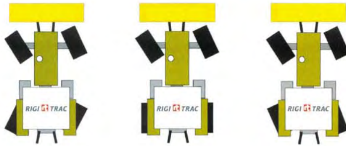
Fig. 2 Steering modes: all wheel, front wheel and crab steer (f.l.t.r.).
