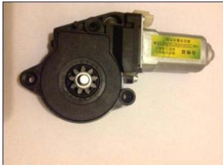
Figure (a): Power Window Motor Figure (b): Torque relation
