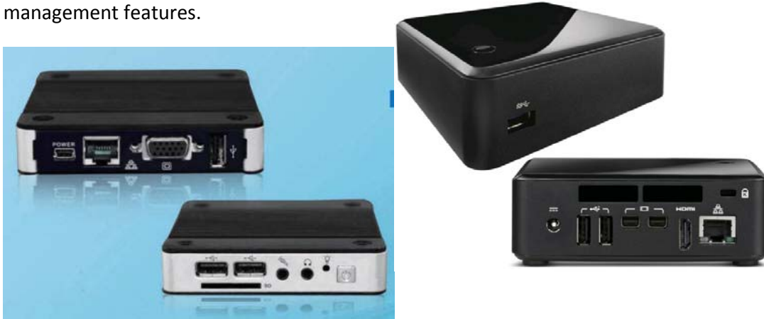
Figure 3.23: eBox and NUC PCs. The eBox is passively cooled while the NUC has a fan to keep the processor cooled.
