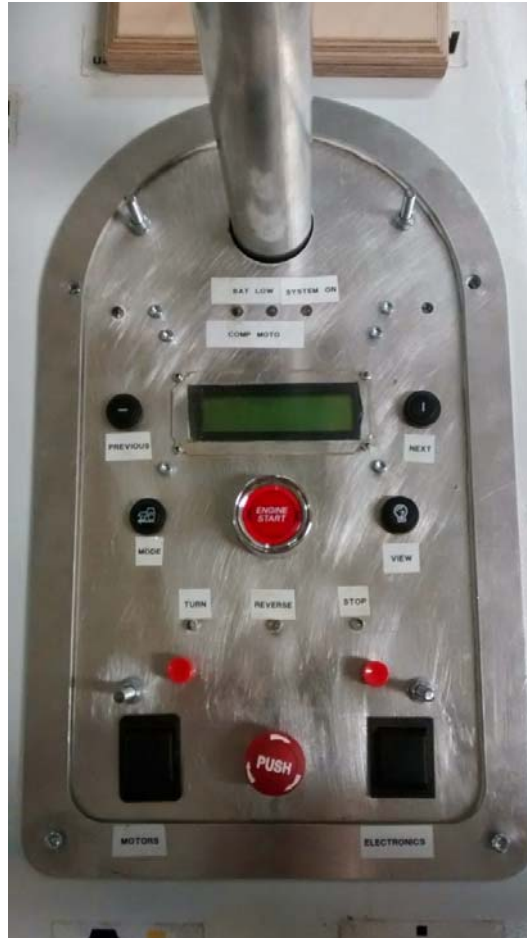
Figure 3.33: Local User Interface. The plate is mounted on tall threaded rods that are attached to the frame of the robot
