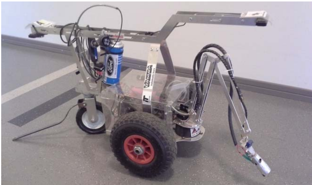
Figure 3.37: The flamethrower trailer used in the freestyle task.
