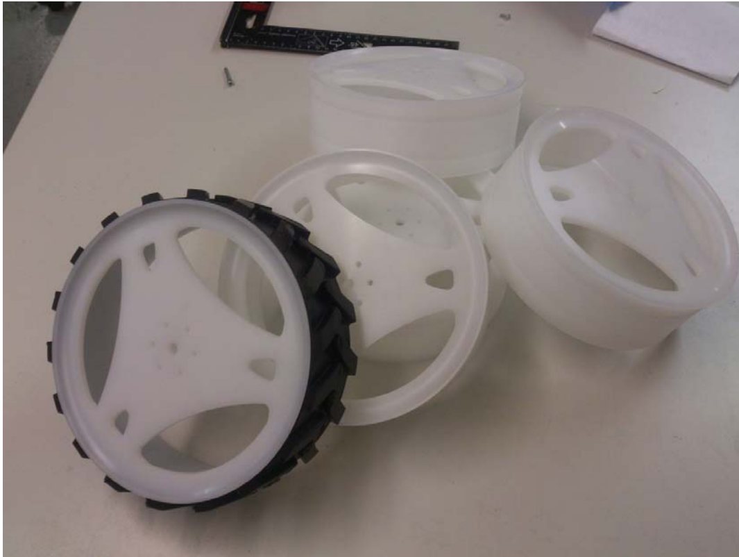
Figure 3.16: The wheels were manufactured from solid pieces of plastic, making them quite expensive to make
