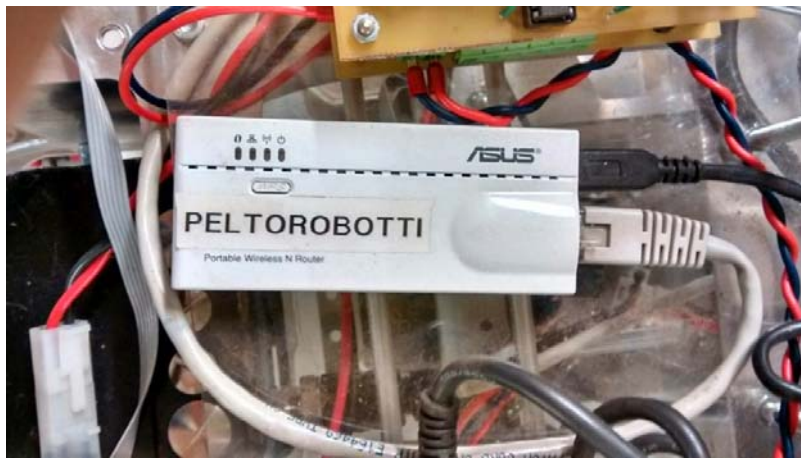
Figure 3.27: The ASUS adapter that was used to provide an access point
