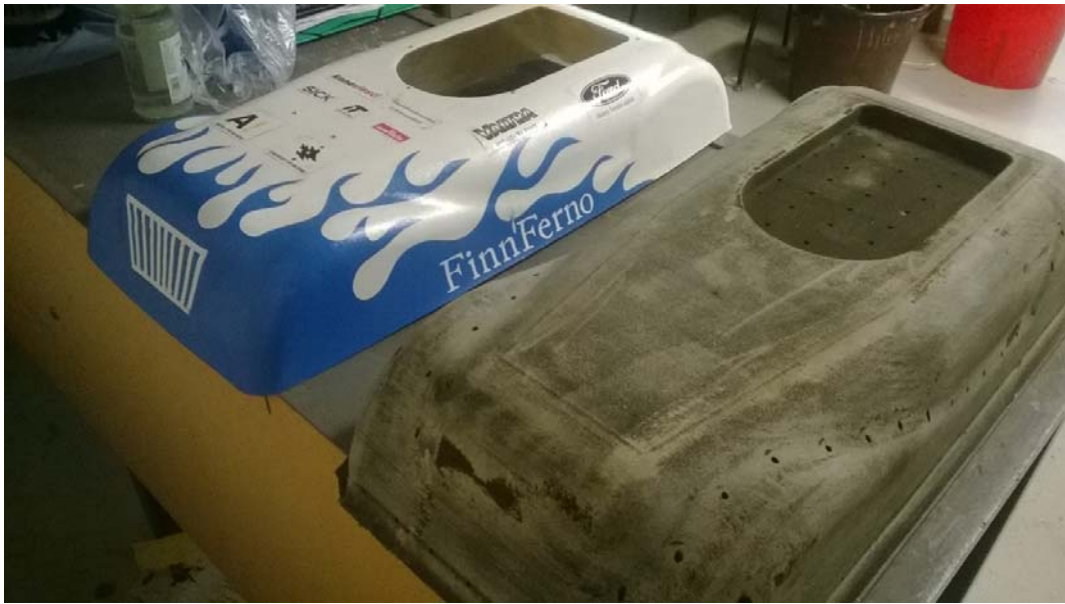
Figure 3.17: Final cover and 3D printed mold
