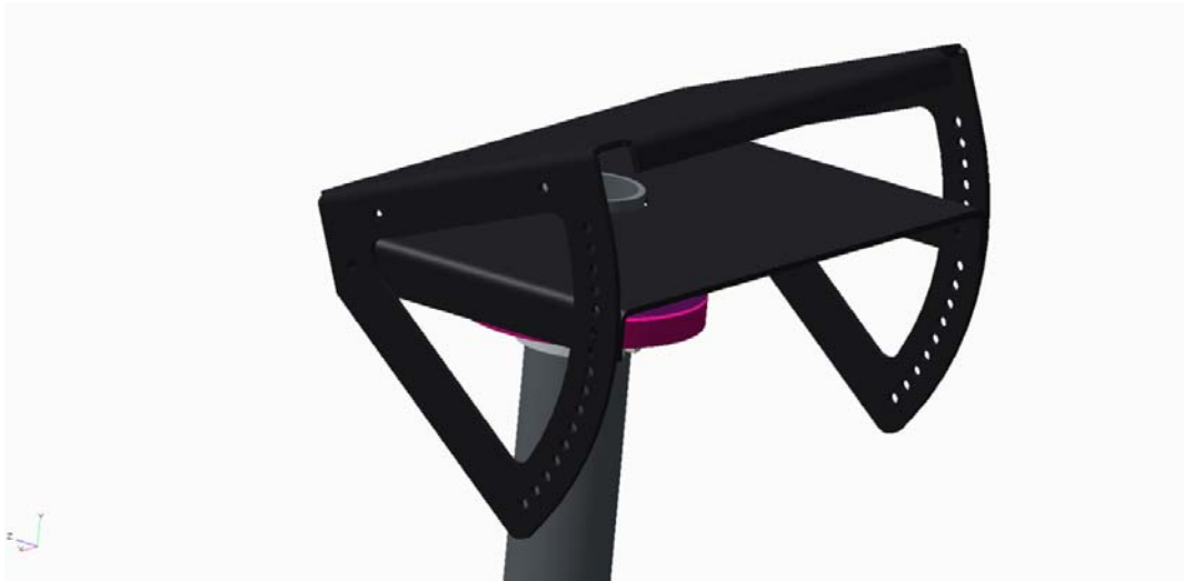
Figure 3.36: Camera mount. The angle of the cameras can be easily adjusted as needed
