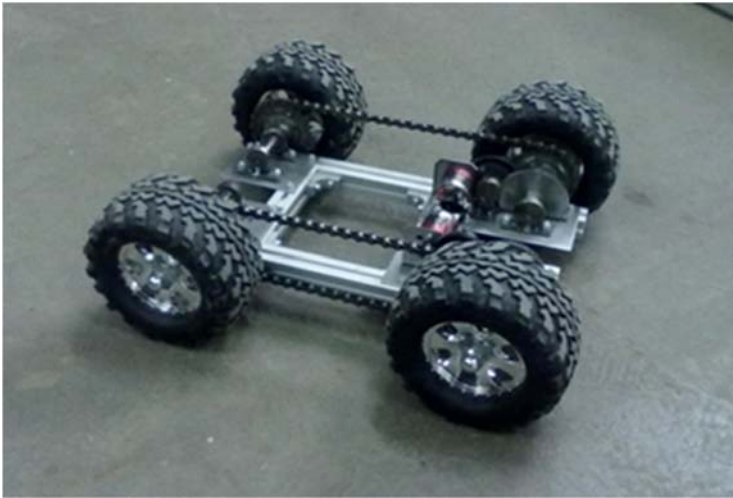
Fig. 2.3 The steering mechanism
