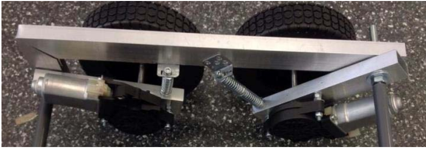
Suspension system for Skid-Steered Vehicle (Gautam 2014)
