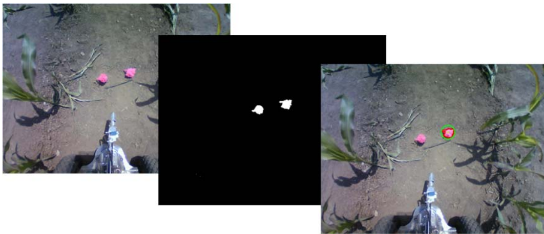
Figure 3.41: Sample picture of trailer's machine vision. Left original picture, middle thresholded and right picture with coordinate point obtained.
