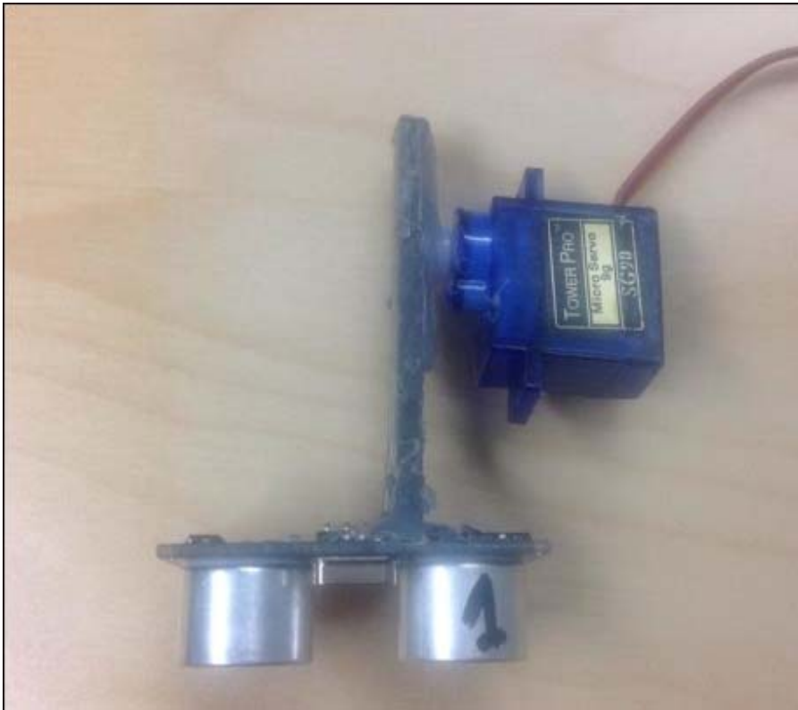
Sonar sensor and servo module (Gautam 2014)
