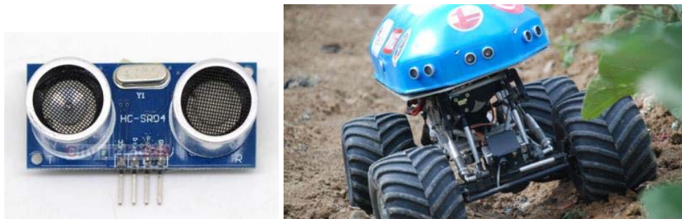
Figure 12 HC_SR04 ultrasonic sensor and application
