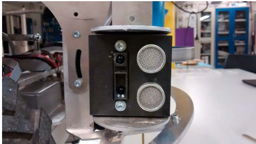
Figure 3.18: The Rangepack module has an infrared sensor (left side) and ultrasonic sensor (right side)
