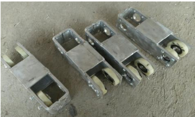
Figure 3. Arms, bush and support of the tires.
