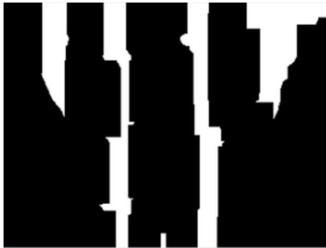
Figure 37: The input image of the machine vision based positioning algorithm. White pixels represent the rows.
