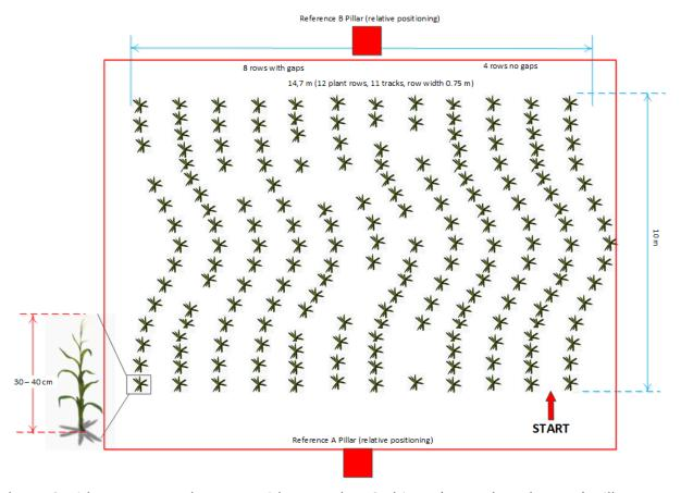
Track 1 to 3 with no gaps, track 4 to 11 with gaps. The 10 objects (5 weeds and 5 cans) will distributed randomly within the field, but not on headlands. The reference point of the coordinate system is in the center of the field (0,0). The pillars will have coordinates as (Xpillar1, Ypillar1) for the upper one and (Xpillar2, Ypillar2) for the lower one.
