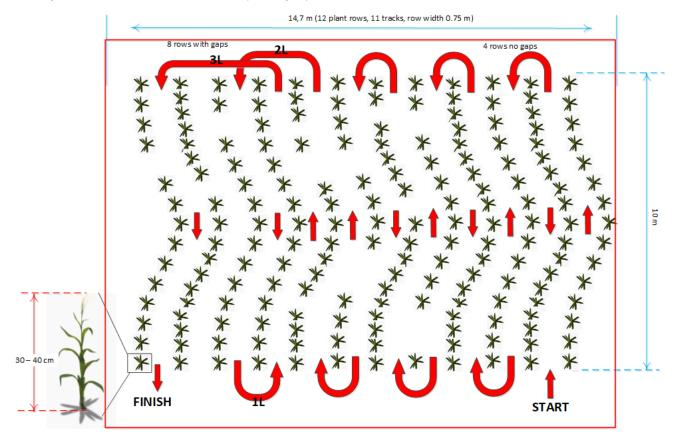
Track 1 to 3 with no gaps, track 4 to 11 with gaps. After track 7 on navigation with pattern 2L (second left), 1L (one left) and 3L (third left) as an example. The headlands are 2 m wide.
